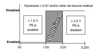
Figure 4: PSON# Signal Characteristics
